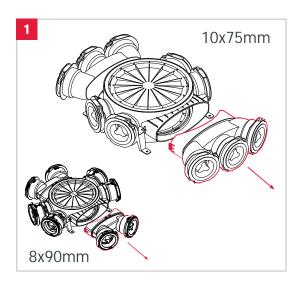
2 Prepare the side connector (sold separately) by cutting the stub end at indentation in order to connect 125 mm pipe. For 160 mm pipe cutting is not required.
