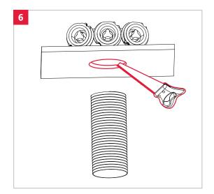
7 After construction works are finished place the disc valve inside the prepared pipe.
