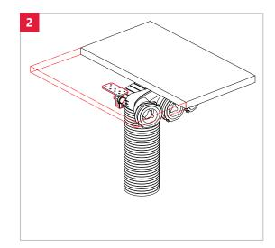
4 Fix the plenum box securely to the ceiling using the holes in the mounting wings by, for example, screws. Diameter of the wing holes is 5,3 mm.
