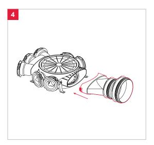
3 Make sure that the seal at the socket is properly placed, if not, correct it. If you notice that the seal is damaged, contact the distributor for a replacement. Dampen the seal to reduce friction.
